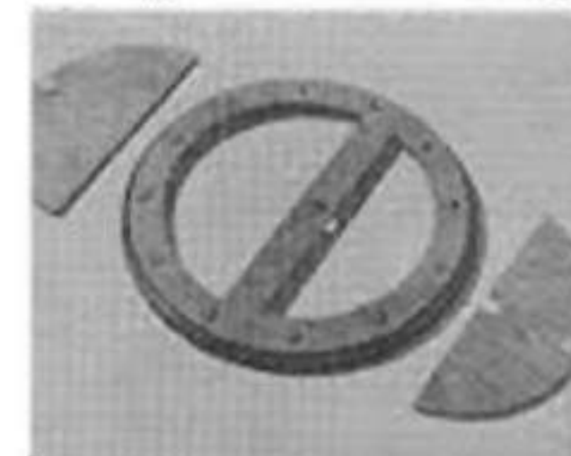
A 12" plywood disc nailed to cut-out can top with upholstery nails makes trap doors and shaft bearing.
