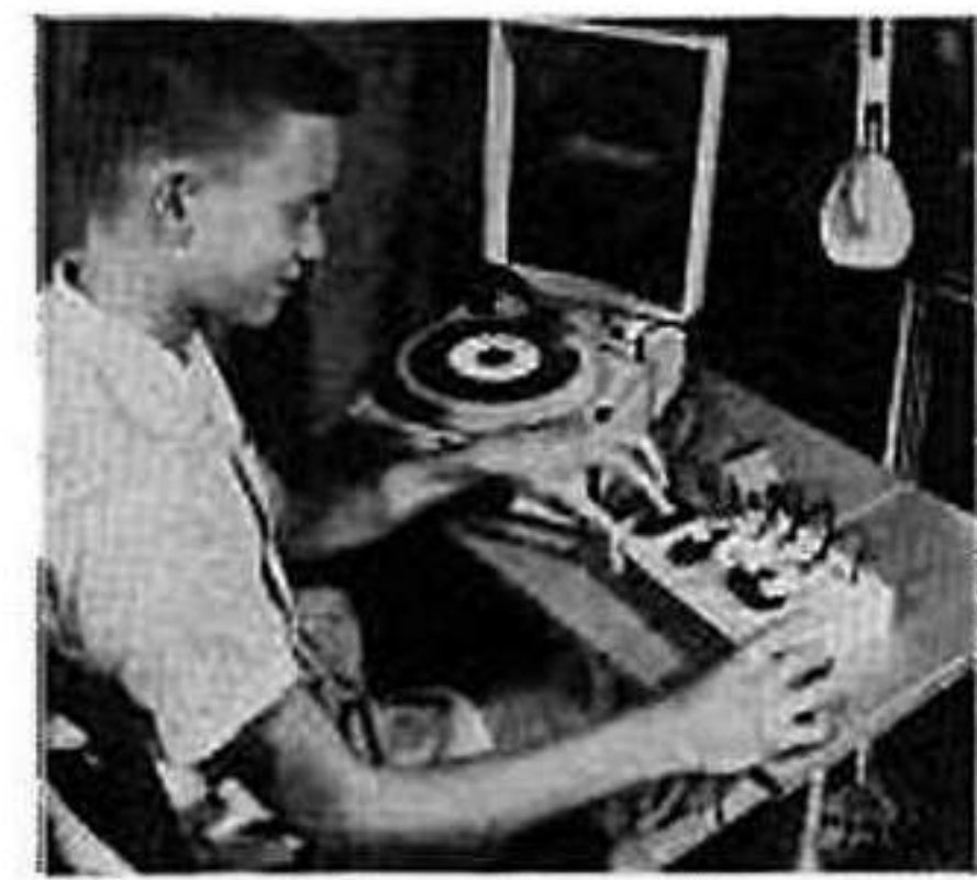
Robot operates by remote control through cable connected to control panel and record player.
