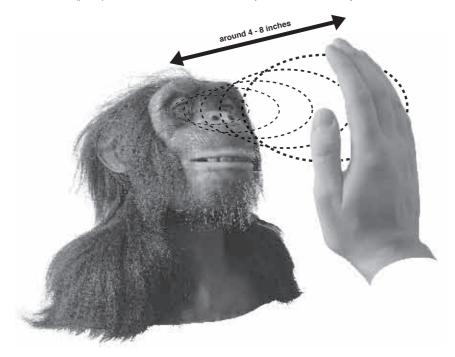
NOTE: The Chimpanzee's Infrared Vision works best at around 4-8 inches from his face. Infrared functions can be affected by bright sunlight, fluorescent and electronically dimmed lighting.
