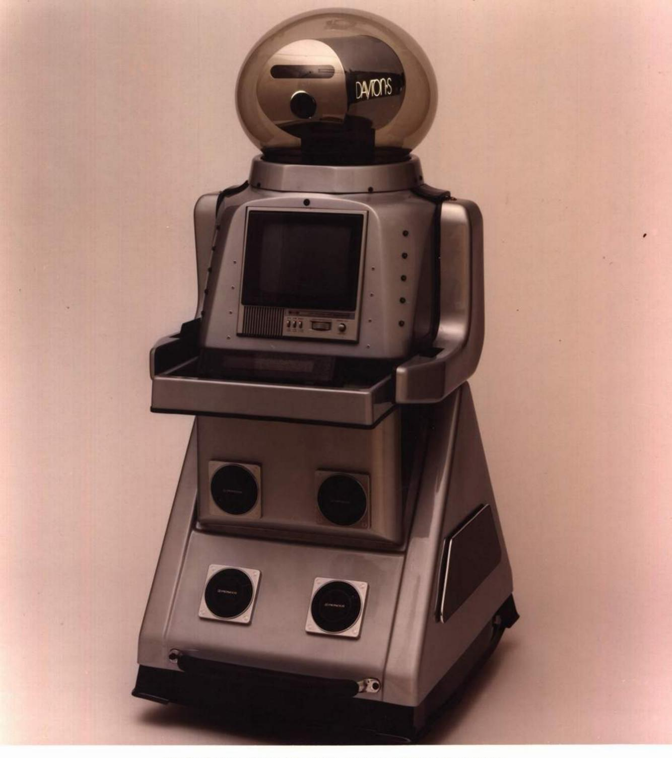
DAYTON'S Department Store, Minneapolis, Minnesota, utilizes a DC-2 robot on a regular basis for promotions. The 4'2" tall robot features a baked-on enamel grey paint job over a sleek fiberglass body with green, flashing L.E.D.'s. Electronics include a 9" color TV in the chest, JVC video camera in the turning head, and a VCR.
