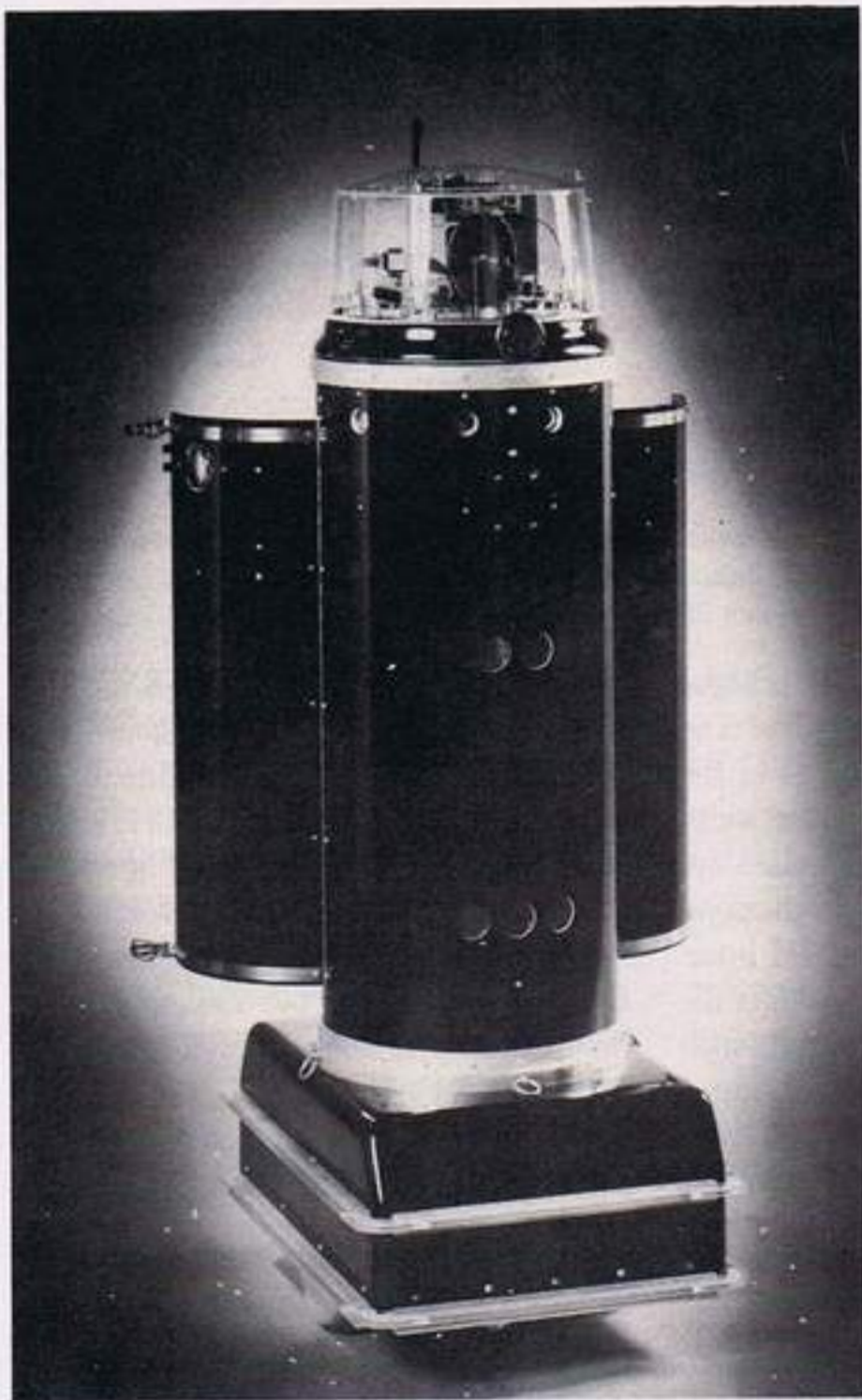
Photo 1. This front view of the prototype robot ROBART II shows the five element ultrasonic sensor array. The upper body case is fabricated from a section of 12 in. plastic irrigation pipe and attaches to the base with four quick-release pins. The parabolic reflector for the long-range near-infrared proximity detector is visible under the plexiglass dome. The photo is courtesy of the Naval Surface Weapons Center.
