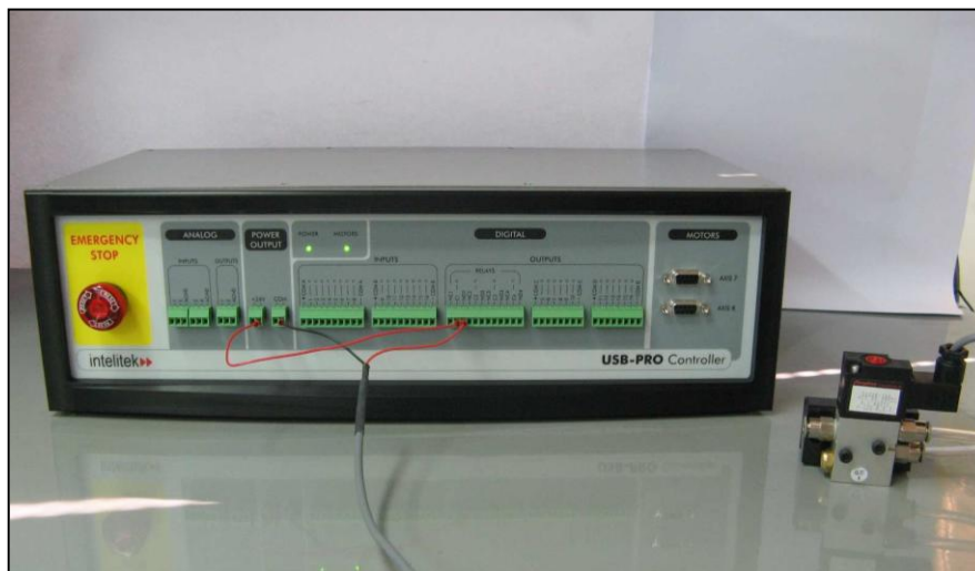
Figure 4-10: Pneumatic gripper valve connection example (front connection)
