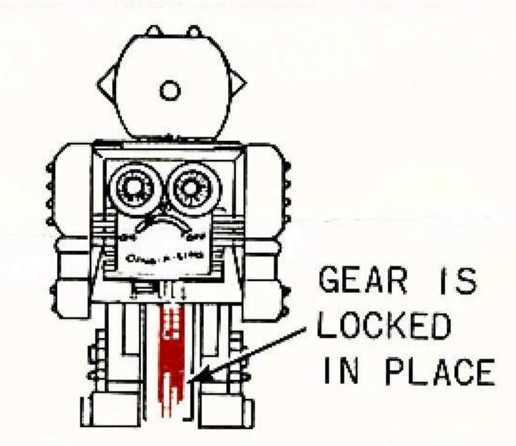
TO MAKE DING-A-LING GLIDE, MOVE SWITCH TO "ON" AND PUSH LEVER ALL THE WAY UP. A GEAR WILL DROP BETWEEN DING-A-LING'S FEET. WHEN LEVER IS ALL THE WAY UP, THE GEAR WILL LOCK IN PLACE.
