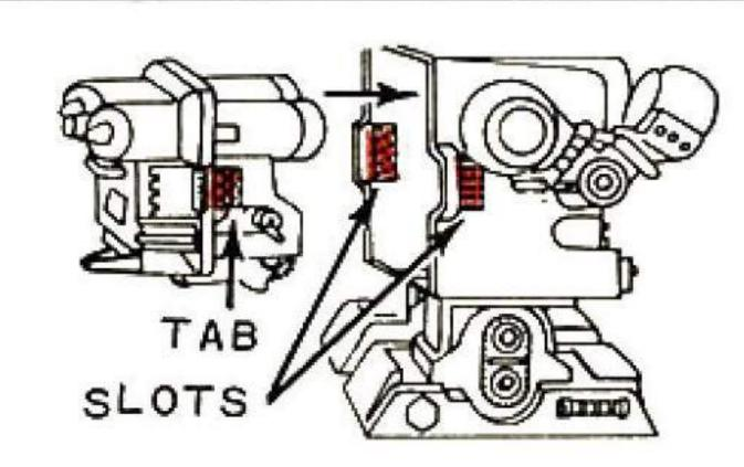
TO INSERT POWER PACK, HOLD AS SHOWN AND PUSH ALL THE WAY IN UNTIL IT CLICKS INTO PLACE. BE SURE TABS OF POWER PACK FITS INTO SLOTS IN DING-A-LING, AS SHOWN.
