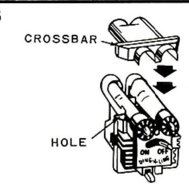
TO PUT ON BATTERY COVER, FIT CROSSBAR INTO HOLES IN POWER PACK AND SNAP COVER INTO PLACE.
