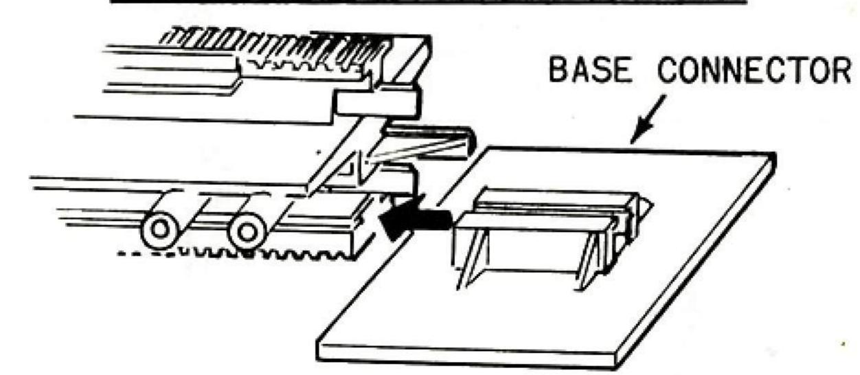
SLIDE TOP OF BASE CONNECTOR ONTO LOWER GROOVES OF SPACE SKYWAY PIECE.
