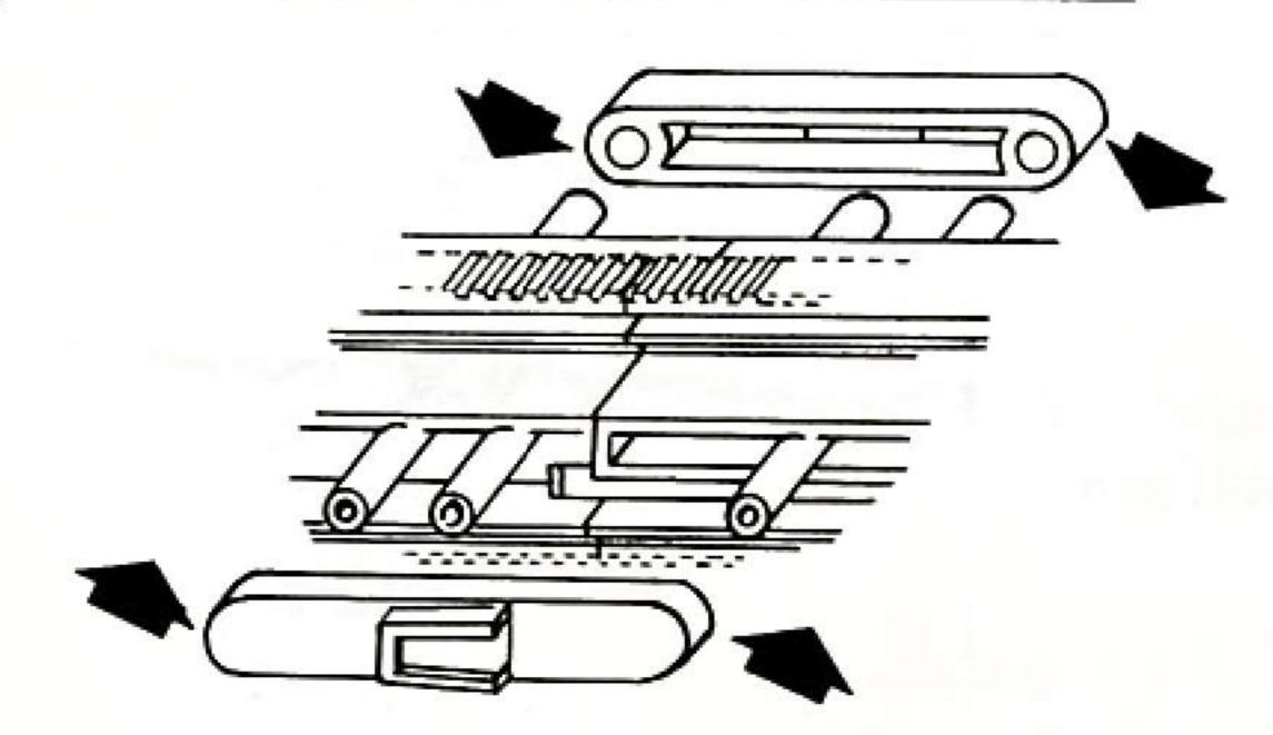
PUSH CONNECTORS ONTO POSTS ON SPACE SKYWAY PIECES, AS SHOWN.
