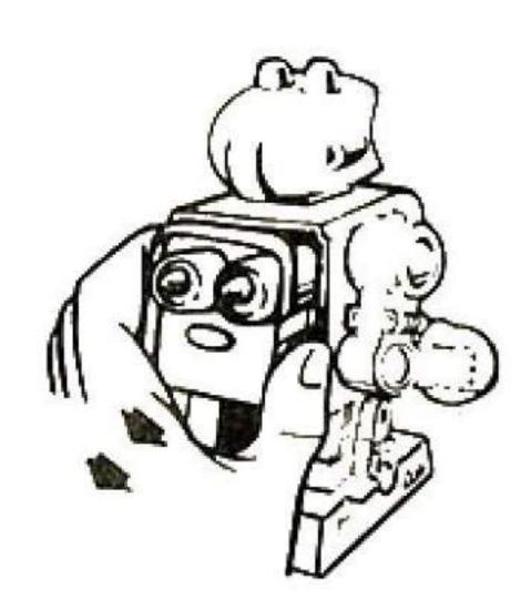
REMOVE BACK FROM DING-A-LING BY PRESSING IN ONE SIDE OF BACK AND LIFTING IT OFF.
