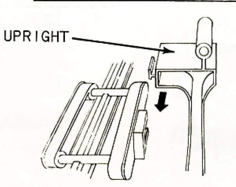
SLIDE BOTH SIDES OF UPRIGHTS ONTO TABS OF CONNECTORS, AS SHOWN.
