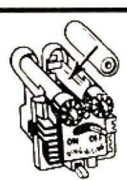
INSERT 2 "AA" BATTERIES (NOT INCLUDED), FOLLOWING DIAGRAM INSIDE BATTERY HOLDER. IMPORTANT: POWER PACK WILL NOT OPERATE UNLESS BATTERIES ARE IS IN THE "OFF" POSITION. LIFT INSERTED PROPERLY AND BATTERY COVER IS IN PLACE.
