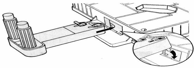
Insert the robot platforms into the holes on the large platform and snap the robot holders into the controllers.
