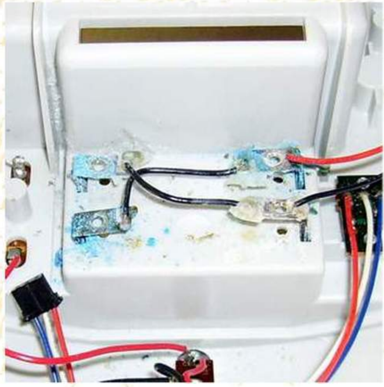
7. Gently pry the battery contacts out.
