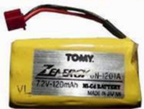
Battery for TXR-002 Tomy Zenergy 6N-1201A 6 Sanyo N-120TA ni-cad cells making 7.2 volts at 120mah.
